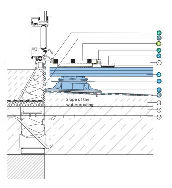
Barrier-free door connection to DIN 18 040 with AquaDrain® VARIO box channel
