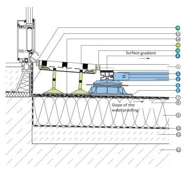
Barrier-free door connection in accordance with DIN 18 040 with diagonally adjustable drain grate that can be cut to length
